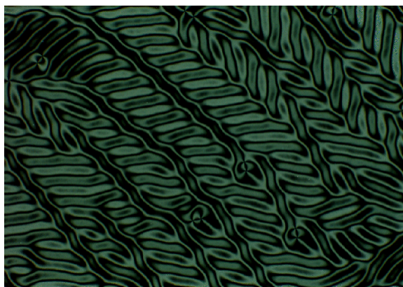
Figure 1: Close up of nematic phase liquid. Image courtesy of Oleg D. Lavrentovich, Liquid Crystal Institute, Kent State University. (2)
