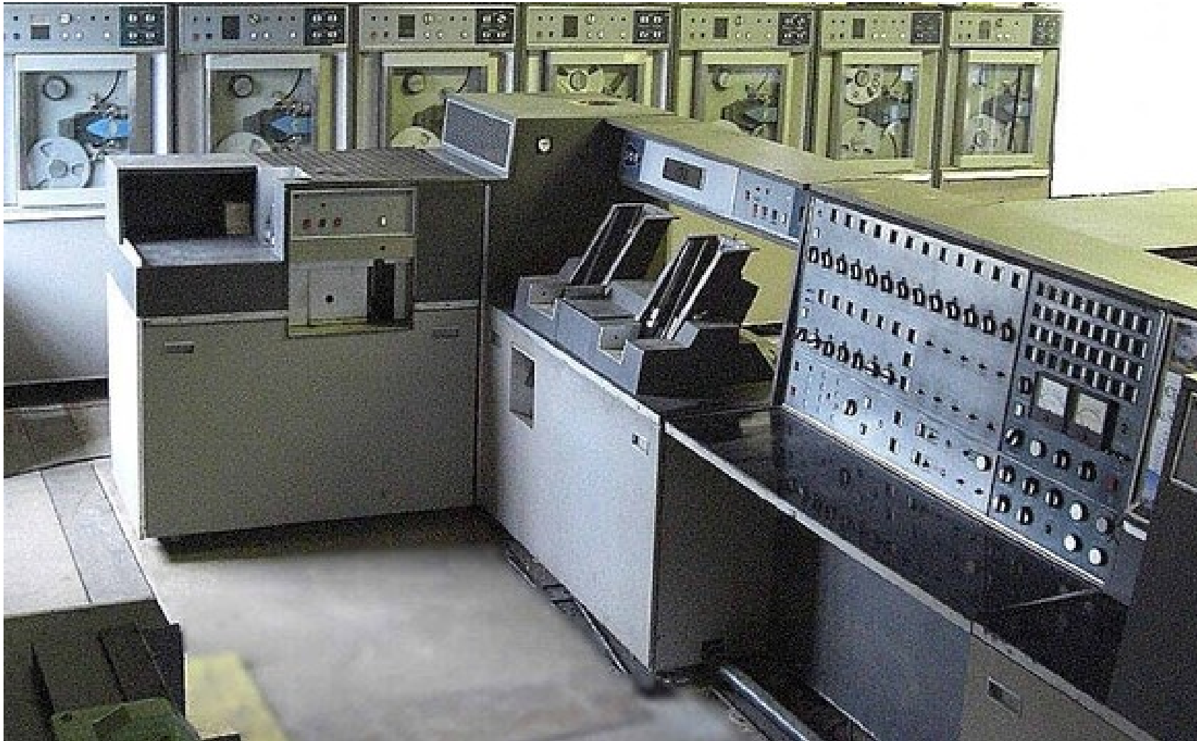
Typical fully transistorized mainframe from UK - ICT 1301.
