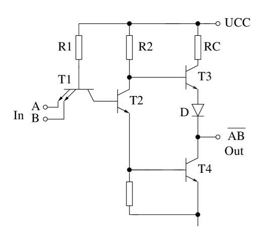
The input is made from the multiemitter transistor. It works in a similar way as diodes in DTL.
