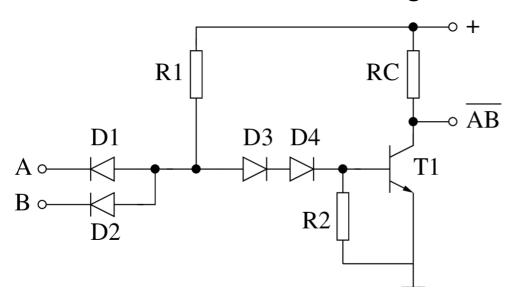
D1 and D3 falls down and the transistor T1 is closed and output is in logical 1. The resistor R2 helps to close transistor and diodes D3 and D4 increase noise immunity. The idea of diodes on input pins is often used to extend some input pins of ICs.
