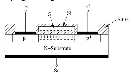
The charged gate can be "cleared" by the UV light. Every erasing process little by little destroys the control gate. The number of erasing and programming cycles is limited.
