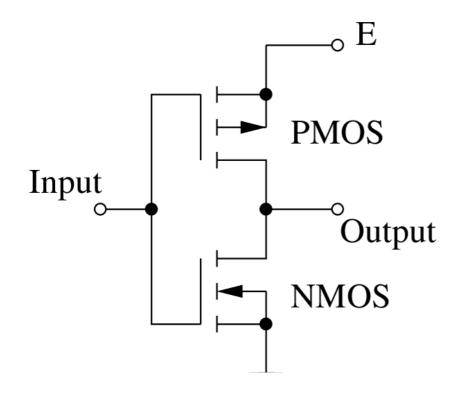
to Gates of PMOS and NMOS transistors. When the Input is in logical 1, the PMOS transistor is closed and the NMOS opened. The output is connected to the ground and its level is in logical 0. And vice-versa. One transistor is always open and the second one is used as high resistance (load) in closed state. The current does not flow in both states from power supply to ground. Gates do not need current either. The consumption of gates is thus zero. This is the main advantage of CMOS!
