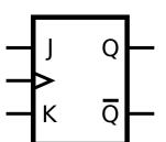
Most versatile of basic flip-flops. Two input behavior plus toggle type behavior.
