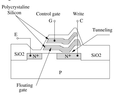
The upper gate is used to control the programming process, the Floating gate stores charge and creates the conductive channel.
