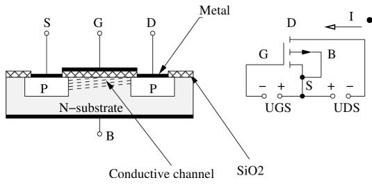
The cross section on the left is a FET with the N channel working in the enhancement mode. The principle of the control is based on the creation and expansion of the conductive channel between the S and D by the voltage on the Gain.
