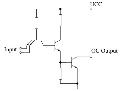
For many application another type of the output is used – **Open Collector**. In the output part there is only the lower transistor and its collector is directly drained out. This output can be used to control the signal on buses (many signals are active in 0) or to switch higher voltage than the supply is.
