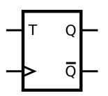
T – Toggle action is useful for counters. Can be constructed from any of the basic flip-flops.
