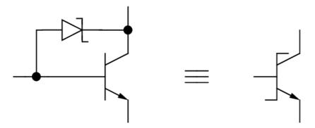
To speed up transistor switching the Schottky diode (metal-semiconductor) can be implemented in circuit between transistor base and collector. The diode does not allow full saturation of the transistor. Thus transistor can close faster.
