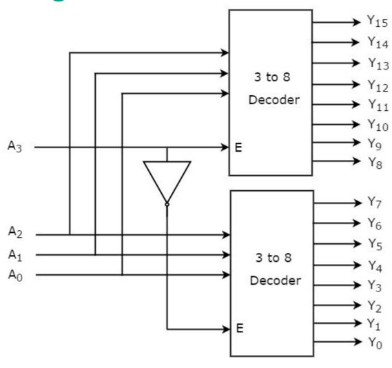
The decoder is a circuit to convert signals combination on input to one unique output.
