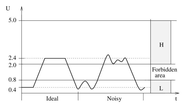
• TTL digital circuits operate in precisely defined voltage levels. You can see them in the diagram above. The high level signal – logical 1 is above 2.0V. The low level – logical 0 is under 0.8V. Forbidden area is between these both levels. When the signal changes its value, it has to pass through this area so quickly as it is possible. The narrowed zone around the forbidden zone – 0.4V - is the zone of the noise immunity.
